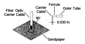
5. Keeping the fiber optic cable end at a right angle to the sandpaper, gently sand the end using a circular motion until the end is smooth (about 15 orbits at 1-inch diameter).
