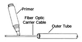
3. Install the fiber optic ferrule over the fiber optic carrier cable and push the stem end into the outer tubing until the flange contacts the outer tubing.
