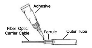
5. Slide the fiber optic carrier cable back and forth for a couple of seconds to promote a good bond to the fiber optic ferrule.
