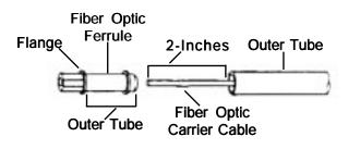
4. Place a small bead of adhesive on the fiber optic carrier cable next to the ferrule.
