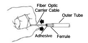
6. Allow a few minutes for the adhesive to set before polishing the fiber optic cable end.
